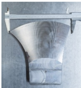
Correct way to measure these dimensions
