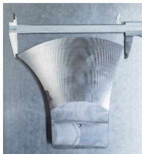
Correct way to measure these dimensions
